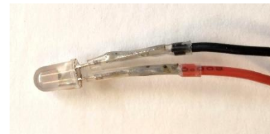
LED soldered to the back wire harness.
