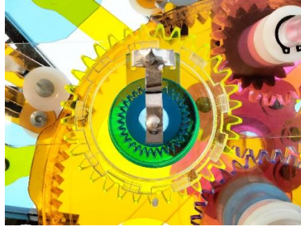
Distributor rotor installed.
