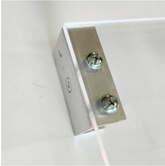
Upper side U-bracket, attached behind the back plate with screws, washers, and nylock nuts.
