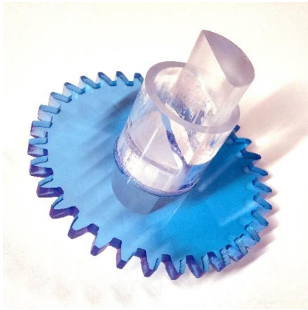
Middle driveshaft with gear33.
