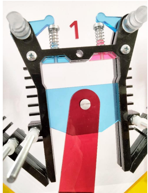
Cylinder with piston, valves, and valve pushers installed.
