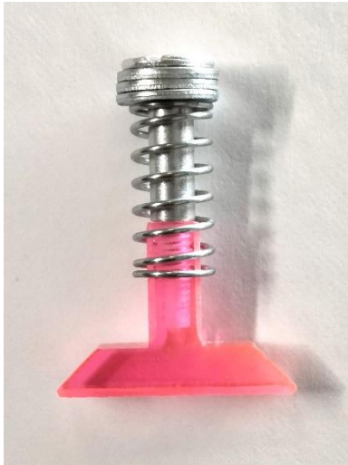
Valve assembly with stem length adjustment washers.
