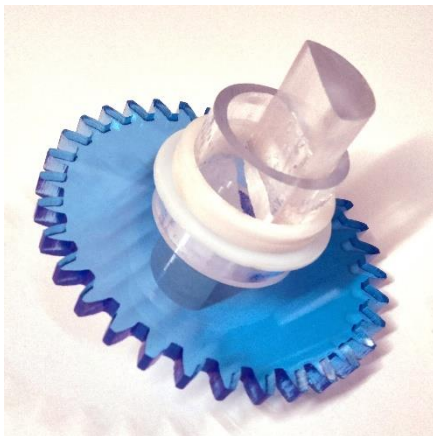
Middle driveshaft with gear33. A shaft sleeve (clear), a spacer ring, and bushing rings are installed.
