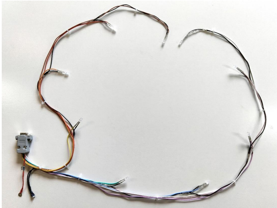
Back wire harness with two main branches and nine LEDs.
