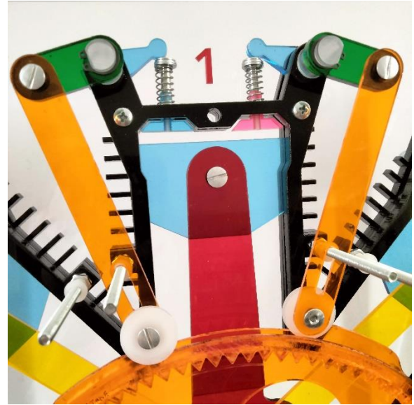
Pushrod assemblies, installed.
