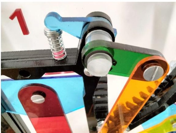
Rocker arm, spacer sleeve, and snap ring, installed. (Installing the rocker arm completes the rocker-pusher assembly.)
