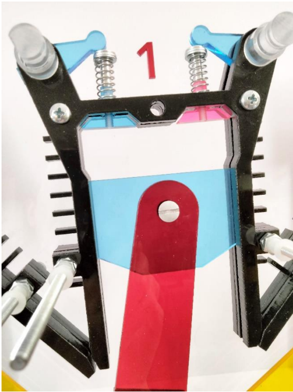
Cylinder with piston, valves, and valve pushers installed.
