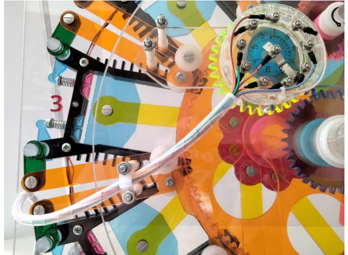
Distributor-cap-&-cable assembly, installed.
