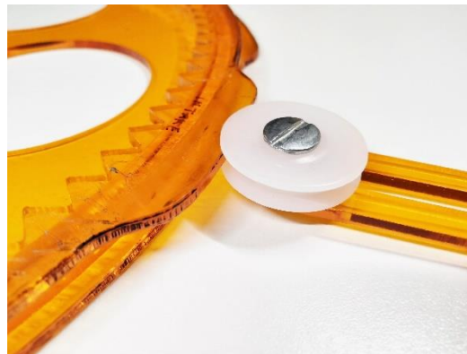
Cam follower (grooved wheel) on cam track.
