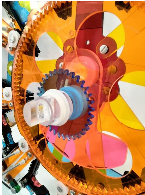
Middle driveshaft with gear33 installed. A shaft sleeve (clear), a spacer ring, and bushing rings are installed in preparation for installing the front plate.
