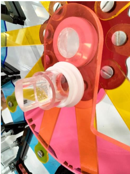
Spacer ring and bushing rings installed in front of the crank front, in preparation for installing the cam disk.
