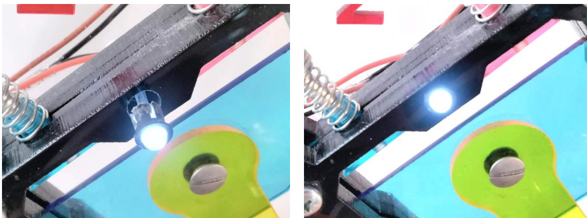
LED pulled forward to install the plastic LED holder.
