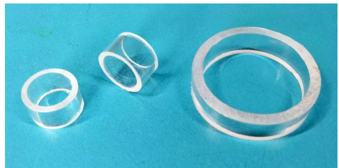
Sleeves, cut from acrylic tubes.
