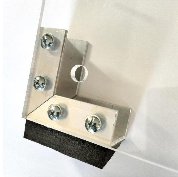
Bottom and lower side U-brackets, attached behind the back plate with screws, washers, and nylock nuts.
