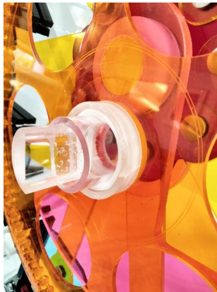
Cam disk installed, with the hub around the bushing rings.
