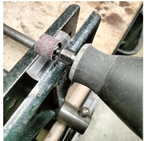
Grinding a D-shaft using a handheld rotary tool with a sanding drum, and a vise.
