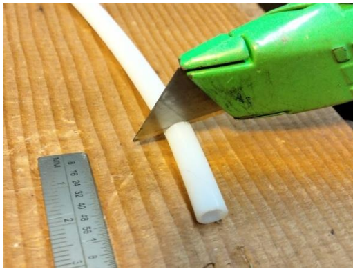
Making a sleeve by cutting plastic tubing using a razor knife.
