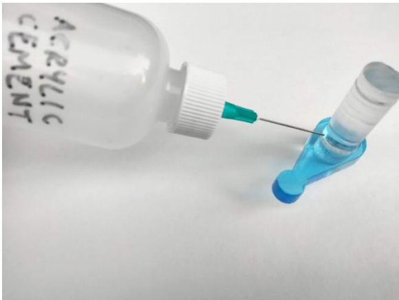
Cementing acrylic parts with a needle applicator.
