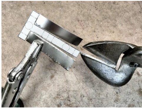
Cutting the T-shaped contacts strip with metal snips, using the paper template as a guide.
