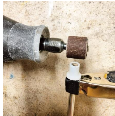
Sanding a sleeve to shorten it and to square the end.
