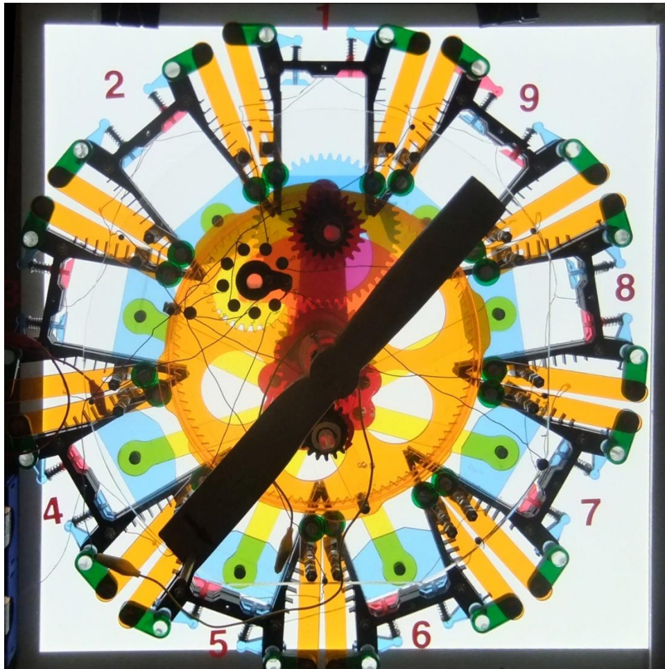
Wes's first complete radial engine model 1, with the mechanical parts and the electrical wiring (2018). [Photo by Wesley Moore.]
