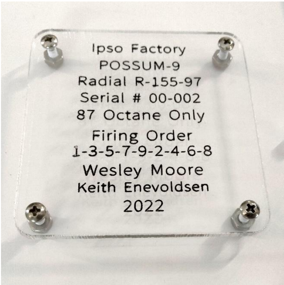
Plaque for model 2 with laser-scored lettering.
