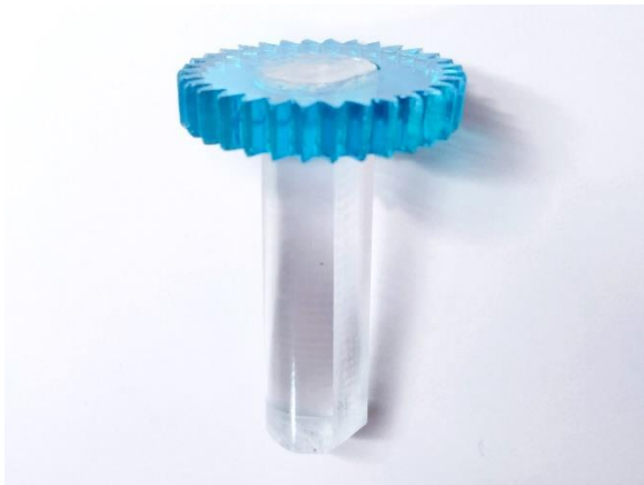
Rotor spline connector with D-shaft.
