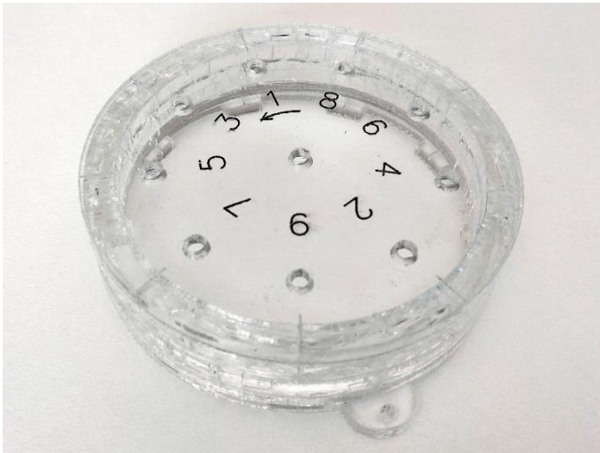
Distributor cap with lid, wall, and twist connector all cemented together.
