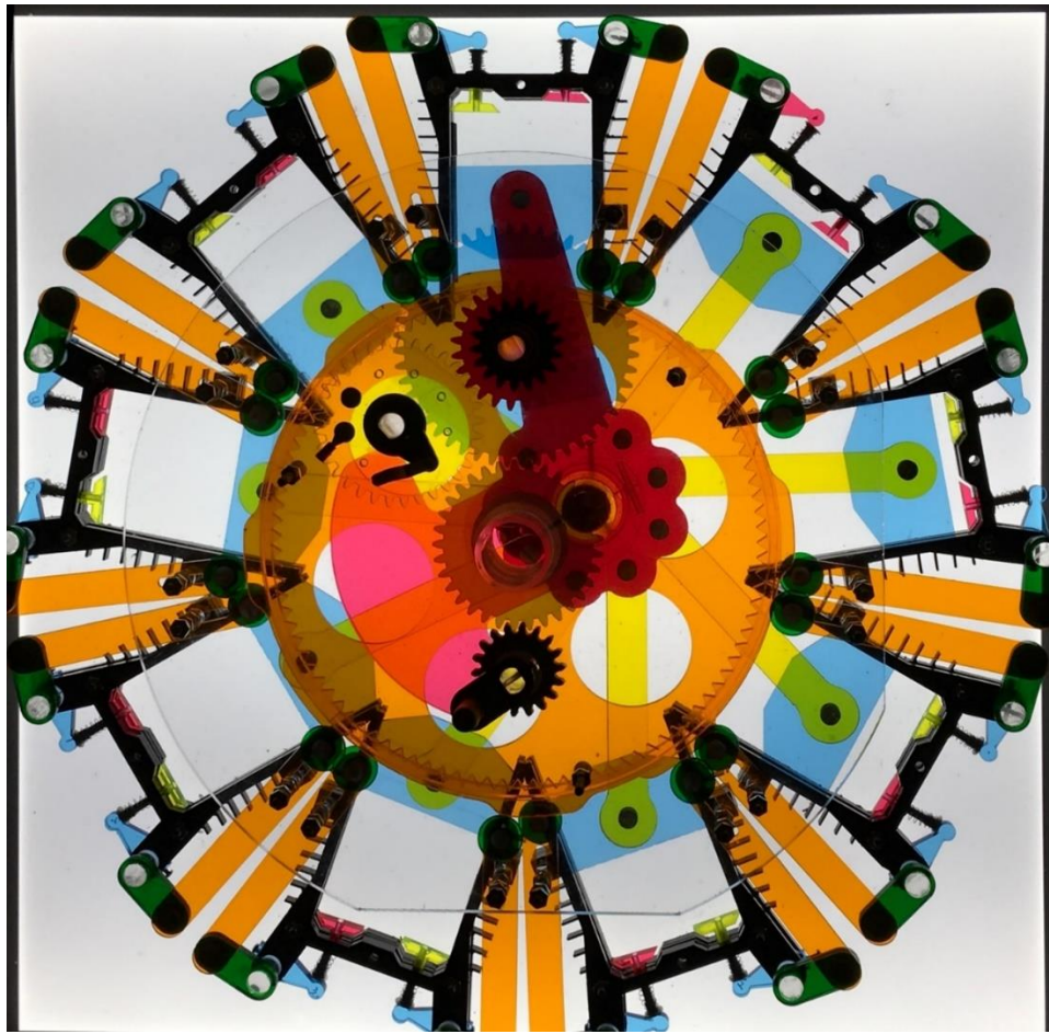
Wes's radial engine model 1, with the mechanical parts, but not the electrical wiring. [Photo by Wesley Moore.]
