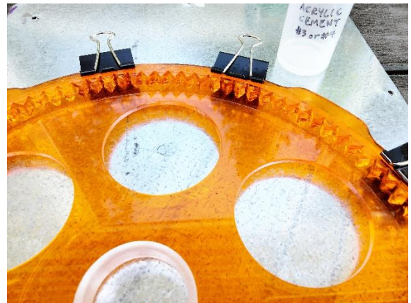
Clamping and cementing the layers of the cam disk.
