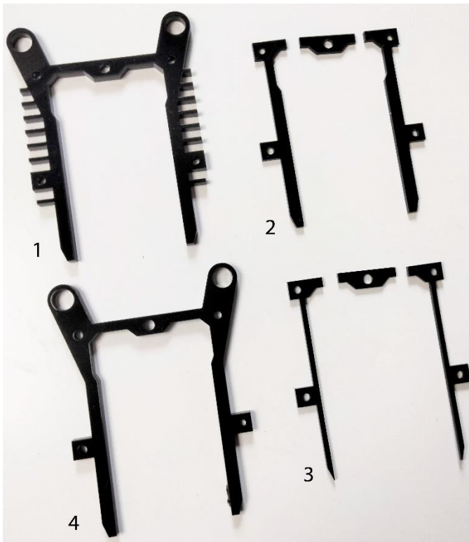
Cylinder layers: (1) back, (2) middle-back, (3) middle-front, and (4) front. After laser cutting, before cementing.
