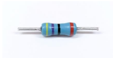
Resistor (47 \Omega , 1/2 W).
