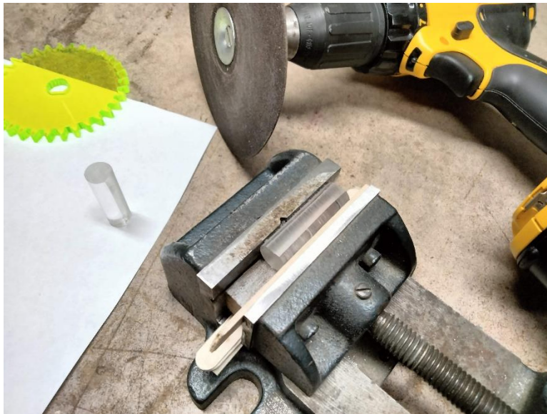
Grinding a D-shaft using a disc sander, vise, blocks, and shims.
