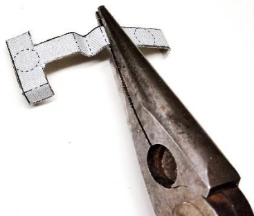
Bending the metal strip with needle-nose pliers, using the paper template as a guide.
