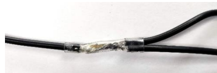
Y join of three negative wires.
