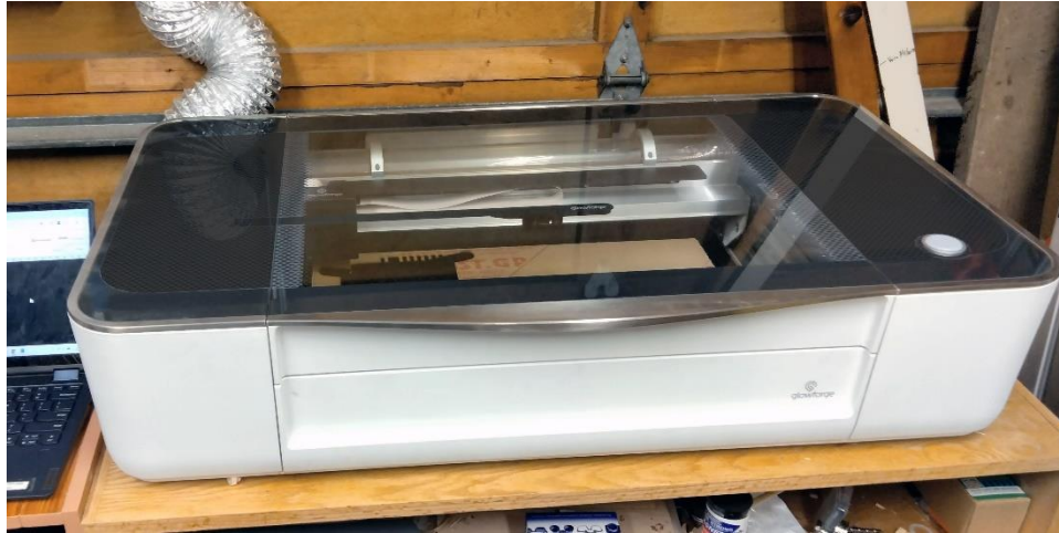
Glowforge 40-watt CO 2 laser cutter.
