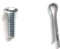
Distributor cap lock screw or lock pin.
