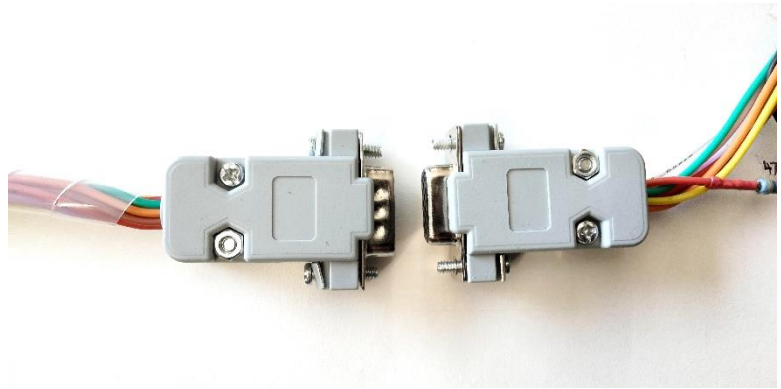
Cable connectors (D-Sub DE-15) on front cable (left) and back wire harness (right).
