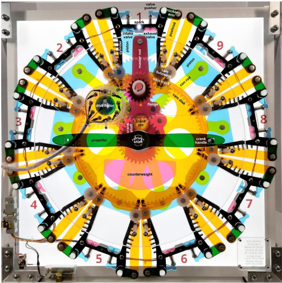
Radial engine model, with parts labeled.
