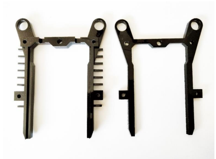
Cylinder back part, after cementing, (left) and cylinder front part (right).
