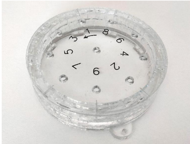
Distributor cap with lid, wall, and twist connector base all cemented together.
