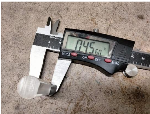
Measuring a D-shaft using electronic calipers.
