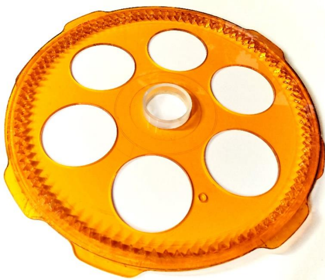
Cam disk with intake cam track (front) and exhaust cam track (back).
