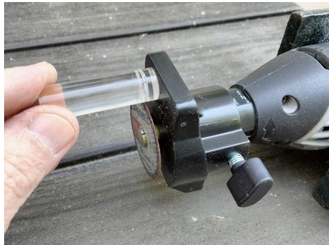
Cutting a snap-ring groove in a D-shaft using a handheld rotary tool with a cutting wheel and a guide
