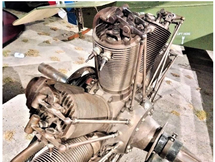
Clerget 9B radial engine, showing cylinders, pushrods, rocker arms, valve springs, and spark plugs.
