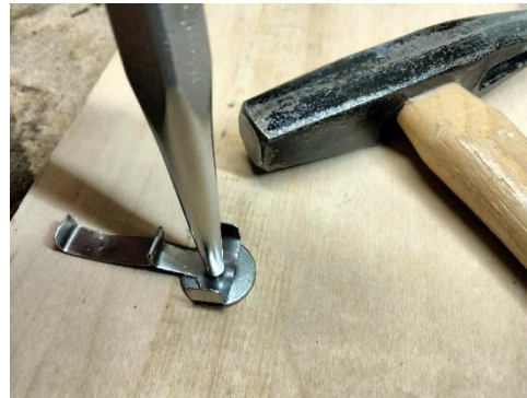
Hammering bumps at contact points, using a hammer, center punch, and washer.
