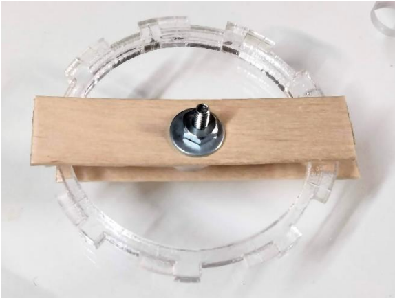
Clamping and cementing the twist connector inner ring to the front plate.
