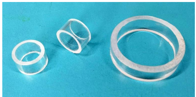
Sleeves, cut from acrylic tubes.
