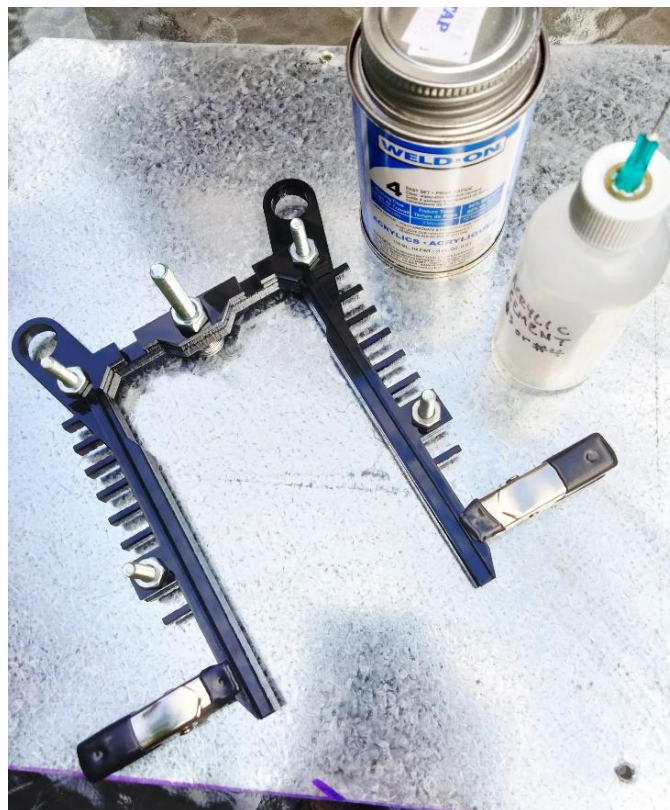
Cementing the layers of the cylinder back part. Use screws, nuts, and clamps to align and clamp the pieces. Apply acrylic solvent cement to the edges after clamping.
