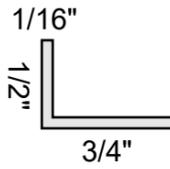
Legs and crossbars are cut from aluminum L-angle 3/4" x 1/2" x 1/16" (or L-angle 3/4" x 3/4" x 1/16").
