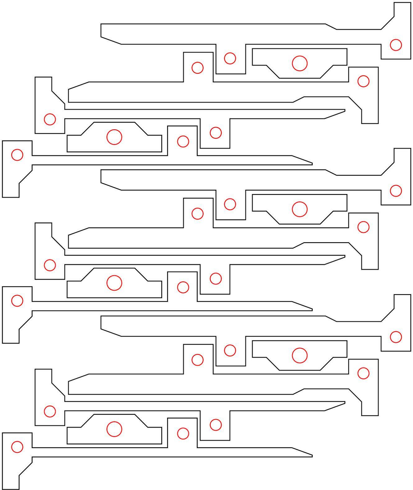
**Cylinder mid-front and mid-back parts — laser template**
